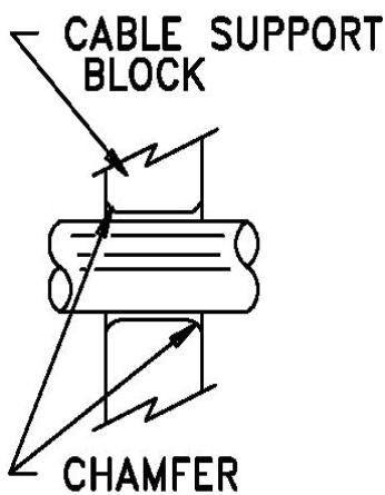
**Chamfered Bore—** The cable bores on our cable support blocks are chamfered to prevent any undue stress on cable insulation. The cable bore is machined with a smooth radius on each side of the bore to prevent the cables from coming into contact with a
